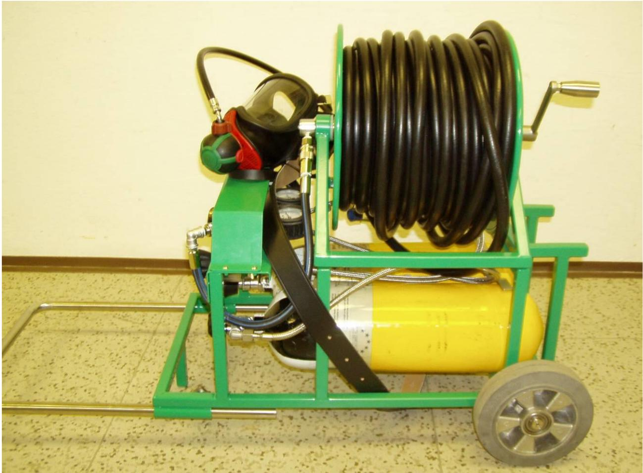
**Appendix A.2 Front view of the AUER DSL-P air apparatus**
